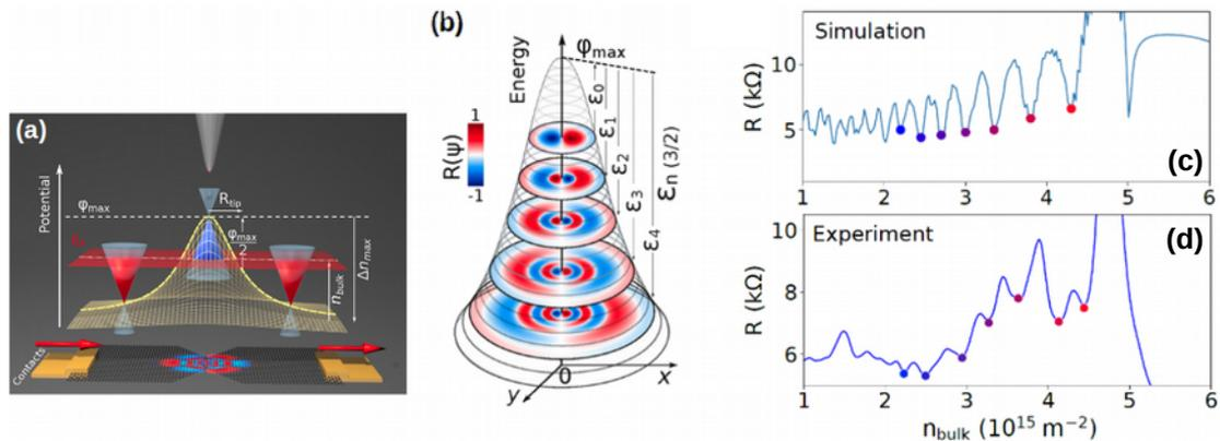
Figure 1: **(a)** Model of the considered whisperitronics device: a polarized AFM tip is scanned above a constriction etched in a graphene device. **(b)** Wave function corresponding to the WGMs with angular momentum  $m = 3/2$ , for its different resonant energies. **(c,d)** Resistance of the device as a function of bulk carrier density, *i.e.*, when tuning the back-gate voltage. The tip is placed above the center of the constriction.
