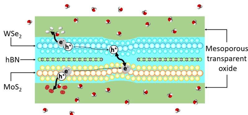
Figure 1: Schematic representation of the SWS system. The active core is based on a  $\text{MoS}_2/\text{hBN}/\text{WSe}_2$  vdWH and a  $\text{MoS}_2/\text{WSe}_2$  vdWH. The former enables the carrier generation and the electrochemical reactions and the latter ensures the extra carriers recombination. A transparent mesoporous oxide supports and protects the active core.
