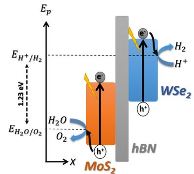
Figure 2: Sketch of the band diagram in the first region where  $\text{MoS}_2$  and  $\text{WSe}_2$  are isolated by hBN.  $E_{\text{H}^+/\text{H}_2}$  and  $E_{\text{H}_2\text{O}/\text{O}_2}$  are respectively the reaction potentials of the reduction of  $\text{H}^+$  in  $\text{H}_2$  and of the oxidation of  $\text{H}_2\text{O}$  in  $\text{O}_2$ .
