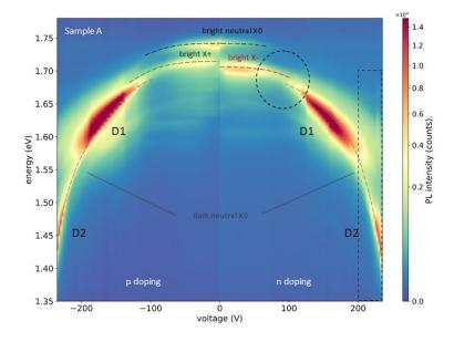
Figure 1: The evolution of excitonic states in WSe2 under strain. A new hybridized state (labelled D1) becomes visible at high strain.
